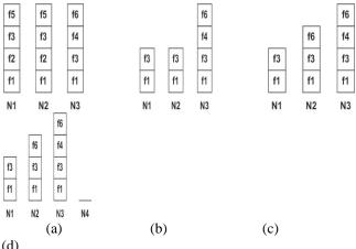
Fig. 1 [1]. An example illustrates the load rebalancing problem, where (a) an initial distribution of chunks of six files  $f_1$ ,  $f_2$ ,  $f_3$ ,  $f_4$ ,  $f_5$ , and  $f_6$  in three nodes  $N_1$ ,  $N_2$ , and  $N_3$ , (b) files  $f_2$  and  $f_5$  are deleted, (c)  $f_6$  is appended, and (d) node  $N_4$ joins. The nodes in (b), (c), and (d) are in a load-imbalanced state.
